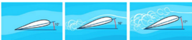
Figure 1: Wing Flow Separation at Stall
