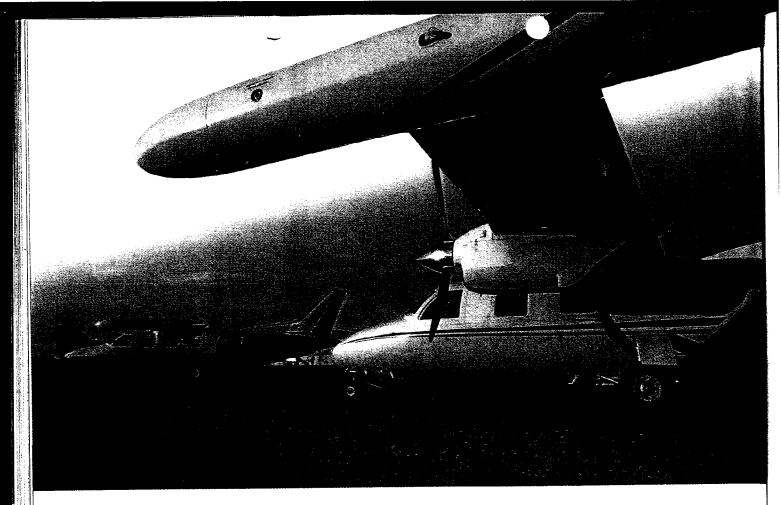
It is fast, dealing with that 300-knot number that has been hard to reach in turboprops. The Solitaire has a top cruise speed of 320 knots, and the long-body Marquise tops out around 305 knots. It is powered by Garrett TPE331 engines. of managed a first
